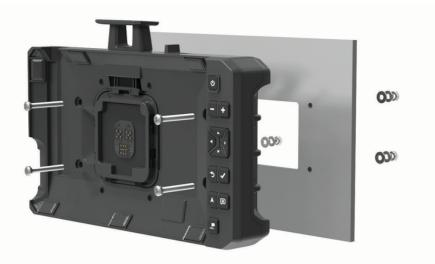
10 Secure the dock to the mounting surface using the appropriate hardware.
