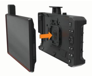
**3** Press down the lock latch ① completely, and slide the lock switch ② toward the latch.
